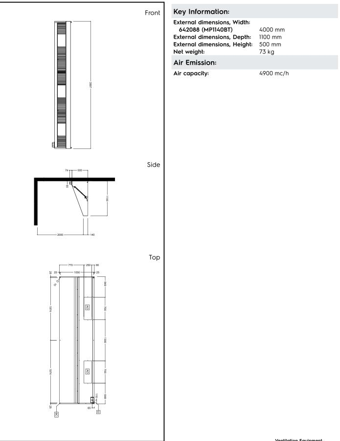
Ventilation Equipment 430 S/S Wall Hood+Filters 4000X1100mm
